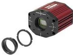
Click to Enlarge Removing the C-Mount adapter and locking ring exposes the SM1 (1.035"-40) threading that can be used for custom assemblies using standard Thorlabs components.
